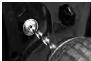
Drill out the original rivets (x3 per woofer) from the factory speaker
