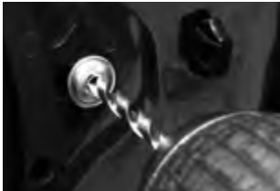
Fig.1 - Drill out the original rivets (x4 per woofer) from the factory speaker
