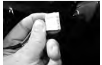
TOYOTA® factory tweeter connector (IS 690TOY)
