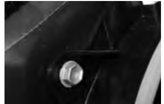
Fig. 2 - Speaker driver screws: IS 690TOY or IC 690TOY
