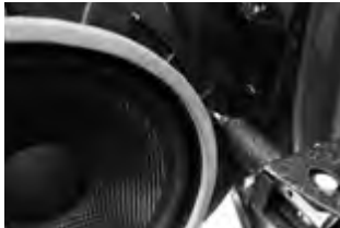
Assemble the Focal speaker using the rivets provided with the IS 690TOY or IC 690TOY kit
